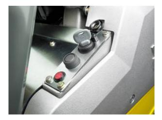
Simply use an ignition key to start the model with electric starter. A loud signal tone prevents inadvertent draining of the battery.
